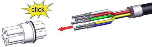
Slide female contacts completely into insulation insert until contacts snap into place.
