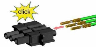
**Slide contact (2) completely into connector shell (3) until contact snaps**
