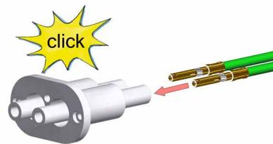
**Slide contact (2) completely into connector shell (3) until contact snaps**
