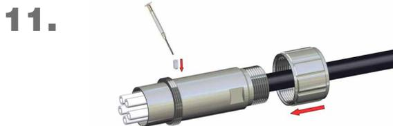
Secure insulation insert (7) with threaded pin (6), then screw joint (4) onto basis (5).
