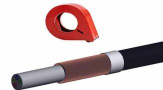
Fix shield braid with tape.
