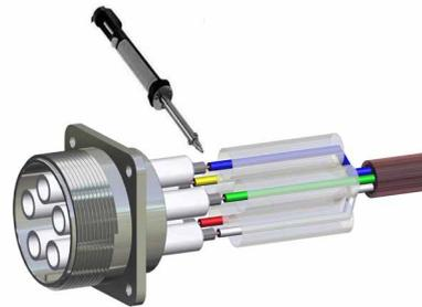
Solder one conductor on each female contact.
