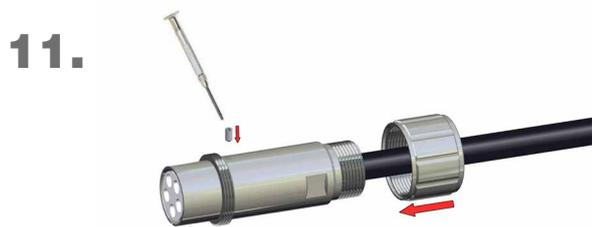
Secure insulation insert (7) with threaded pin (6), then screw joint (4) onto basis (5).
