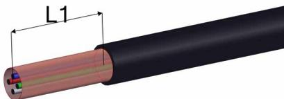
Carefully remove cable jacket (L1 = 28 mm [1.102"])
