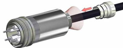
Completely slide seal insert (2) under shield braid into cable gland basis (3).
