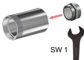
**Screw cable gland basis (3) to housing adapter (4).**
