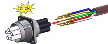
**Slide contacts completely into insulation tubes until contacts snap into place.**
