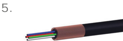
Remove any filling elements from cable
