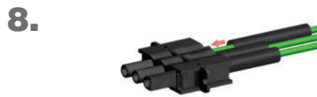
Slide shrinking tube (1) on connector shell (3)
