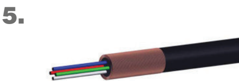
5. Remove any filling elements from cable
