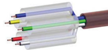
Slide one shrinking tube on each single wire.
