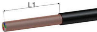
Carefully remove cable jacket (L1 = min. 65mm). ⚠ Do not damage metal shield braid.
