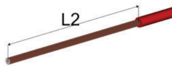
⚠ ONLY when using shielded cable: Remove cable jacket
