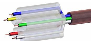
Slide one shrinking tube on each single wire.
