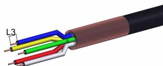
Remove dielectric insulation of single wires (L3 = 5-8 mm [.197" - .315"]).
