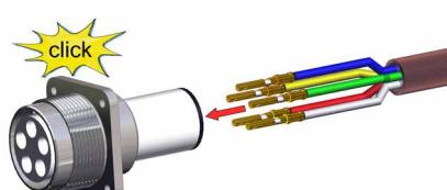
Slide contacts completely into connector shell until contacts snap into place.
