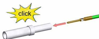
**Slide contact (2) completely into connector shell (3) until contact snaps**
