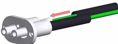
**Slide shrinking tube (1) on connector shell (3)****8.**
