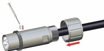
Secure insulation insert (7) with threaded
