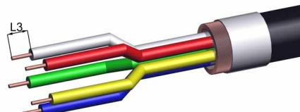
Remove dielectric insulation (L3 = 5-8 mm [.197" - .315"]).
