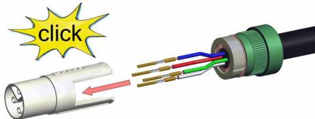
Slide contacts (5) completely into insulation part (6) until contacts snap
