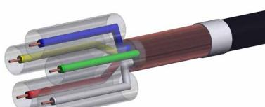
**Place shrinking tubes on single wires.**
