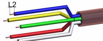
Remove dielectric insulation of single wires (L2 = 5 mm [.197"]).
