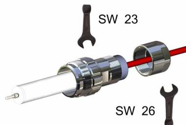
**Screw cap (1) onto housing (3)**
