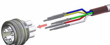
Slide contacts (7) completely into insulation tubes (5).
