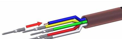
Crimp or solder female contacts (1) on conductor.
