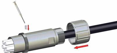
Secure insulation insert (7) with threaded pin (6), then screw joint (4) onto basis (5).
