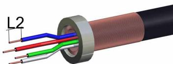
Remove dielectric insulation of single wires (L2 = 4 mm [.157"])
