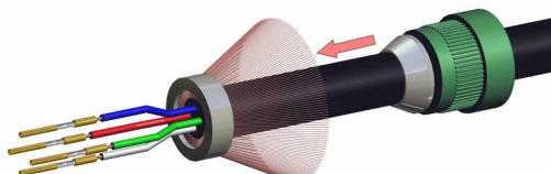
Completely widen shield braid. Push outer cone (3) and clamping rubber (2) under shield braid against inner cone (4) until shield braid clamps between outer cone (3) and inner cone (4)
