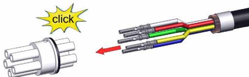
Slide female contacts completely into insulation
