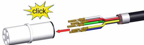
Slide female contacts (1) completely into housing basis (7) until contacts snap into place.
