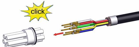
Slide male contacts (1) completely into insulation tubes (7) until contacts snap into place.
