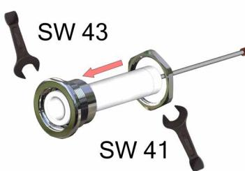
Screw on counter nut and tighten
