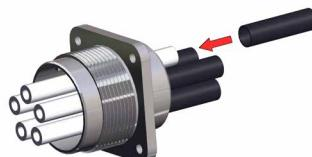
Put shrinking tubes on insulation tubes on back of connector housing.
