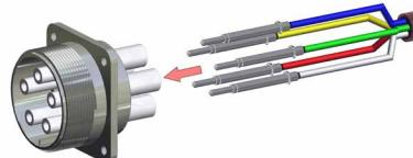
Slide single wires completely into insulation tubes.
