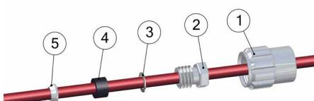
Place screw joint (1), screw (2), washer (3), clamping rubber (4), outer cone (5) on cable
