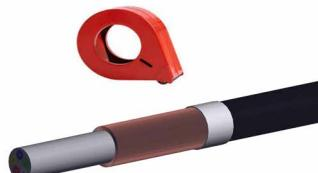
**Fix shield braid with tape.**
