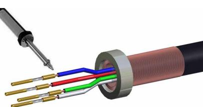
Crimp or solder one contact (5) each on every conductor
