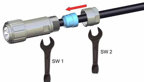
Insert sealing (3) completely and screw
