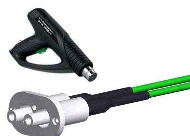
**Shrink tubes - shrinking temperature 110°C****9.**
