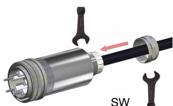
Screw cable gland cap (1) to cable gland basis (3).
