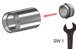
**Screw cable gland basis (3) to housing adapter (4).**
