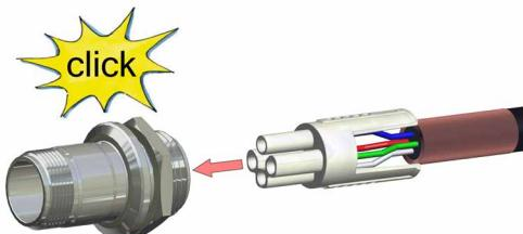
**Put insulation part (2) into housing (3)**
