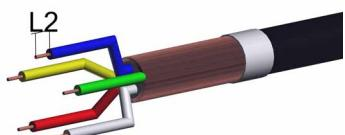
**Remove dielectric insulation (L2 = min. 5 mm [.197"]).**
