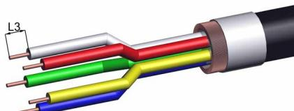
Remove dielectric insulation (L3 = 5-8 mm [.197" - .315"]).
