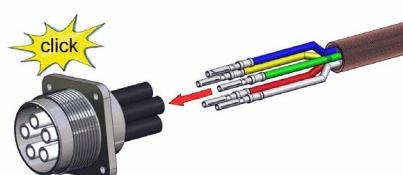
Slide contacts (2) completely into insulation tubes until contacts snap into place.
