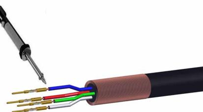
**Crimp or solder one contact (1) each on every conductor**
