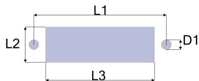
**Panel cut out – feedthrough mounting**
