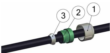
Place cap (1), clamping rubber (2) and outer cone (3) on cable
