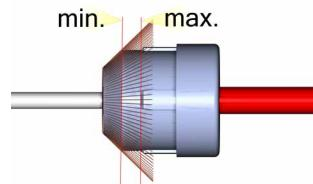
**Make sure shield length is between min.
