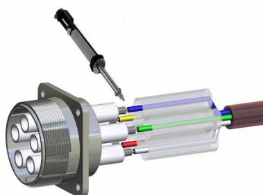
Solder one conductor on each female contact.
