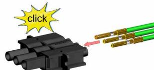
**Slide contact (2) completely into connector shell (3) until contact snaps**
