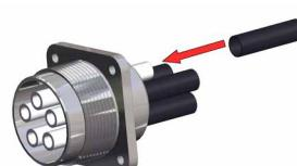
Put shrinking tubes (1) on insulation tubes on rear side of connector housing (3).
