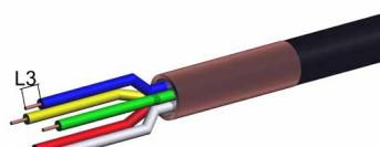
Remove dielectric insulation of single wires ( $L3 = 5-8 \text{ mm } [.197" - .315"]$ ).
