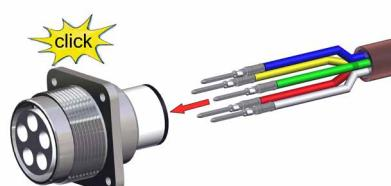
Slide contacts (1) completely into connector shell (2) until contacts snap into place.
